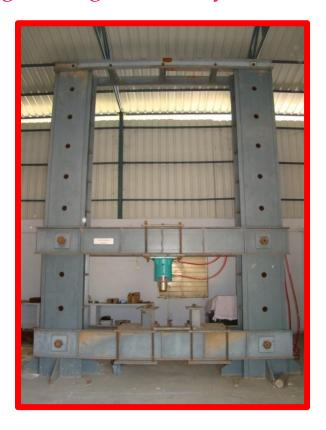
Strength of Materials Laboratory - 400 KN Electronic UTM
